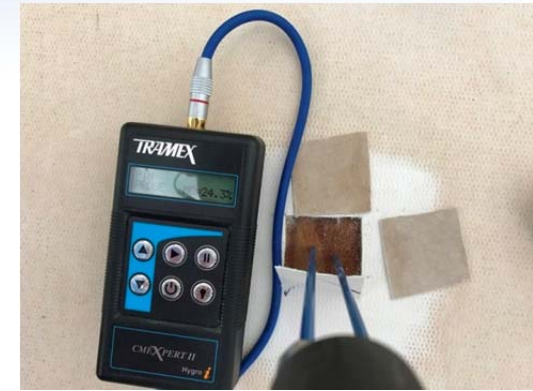
Photo No. 33 – Depicts NMRC moisture meter that detects approximate relative moisture content by electrical conductance. The insulated pin probes pushed into the surface of the plywood measured moisture to be above 24%, which is considered to be fully saturated.
