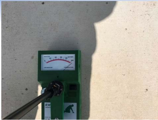
Photo No. 31 – Depicts one of numerous locations measure by NMRC using an electric radio frequency impedance scanner to detect underlying moisture within the system. The meter read over 100 at this location, indicating liquid moisture is present underlying the membrane.
