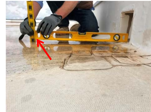
Photo No. 21 – Depicts NMRC Analyst measuring more than one-inch of standing water adjacent to a drainage scupper. Long standing moisture may result in premature deterioration of the membrane due to biological activity acting on the carbon based membrane, and also encourages pressure drive.
