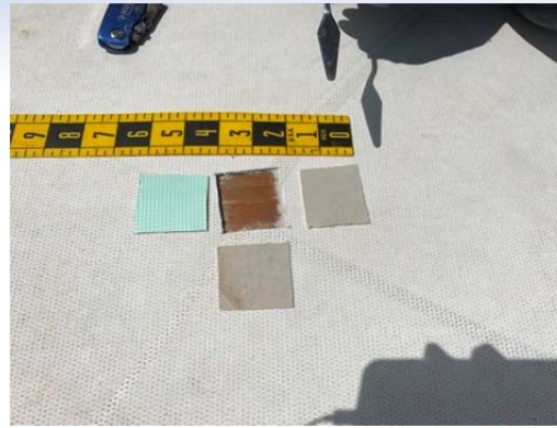
Photo No. 32 – Depicts one of NMRC's test cores. The membrane is installed over two layers of slip sheet directly above a plywood deck. The plywood deck was found to be wet.
